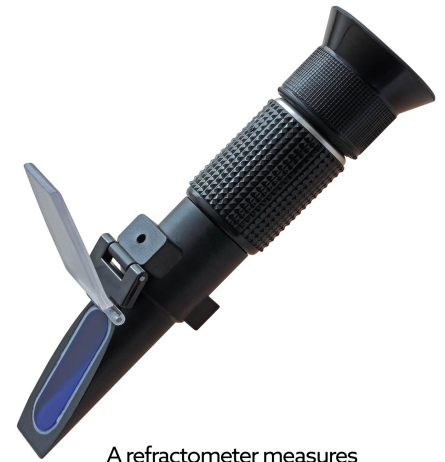
A refractometer measures the specific gravity (or the concentration) of the urine.
